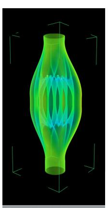
This month shows the inside contour surface of a Heat Exchanger (Condenser) produced by direct metal laser sintering (DMLS). Reconstructed surface contours like this created in Imaris from X5000 Xray CT date are used to compare the geometrical parameters of the printed object to the design. The sample was scanned using the X5000 NSI High Resolution Micro-CT and rendered in 3D using Imaris at the Core Facilities. Image provided by Kazi Fazle Rabbi from the Nenad Miljkovic Group.
