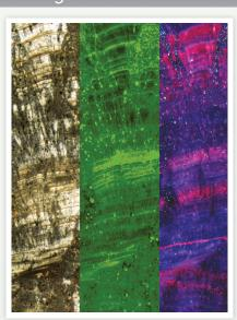
This month's image, "High Frequency Layering in Travertine from the Anio Novos Roman Aqueduct," is courtesy of the Bruce Fouke Lab. The image was taken using the Zeiss Stereolumar v12 microscope.
