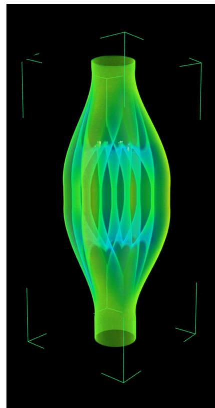
This month shows the inside contour surface of a Heat Exchanger (Condenser) produced by direct metal laser sintering (DMLS). Reconstructed surface contours like this created in Imaris from X5000 Xray CT data are used to compare the geometrical parameters of the printed object to the design. The sample was scanned using the X5000 NSI High Resolution Micro-CT and rendered in 3D using Imaris at the Core Facilities. Image provided by Kazi Fazle Rabbi from the Nenad Miljkovic Group.
